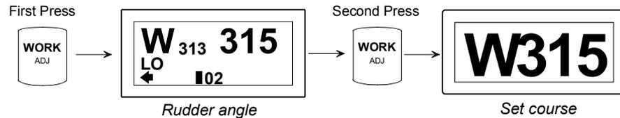
At such incidents some boats may need a rudder off-set when steered by hand. By selecting WORK-mode directly from STBY-mode the rudder off-set is maintained and becomes the TRIM value.
