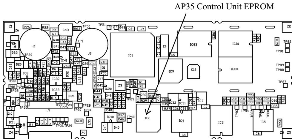
**Figure 5-2 AP35 PCB, component layout**
