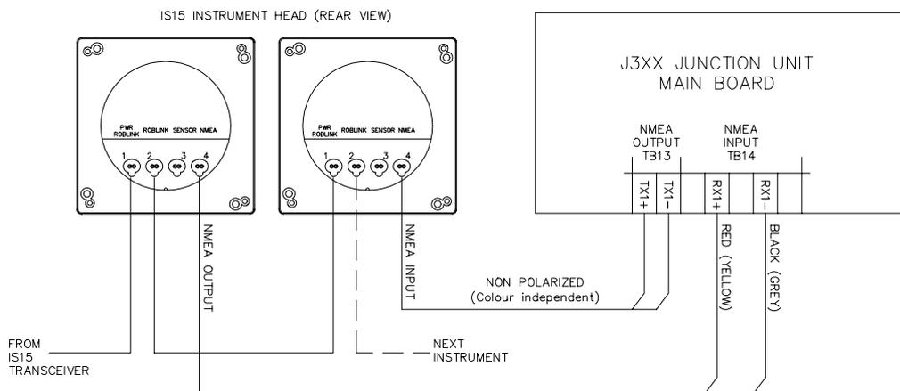
**Figure 4-25 IS15 Instruments / J3XX Connection**
