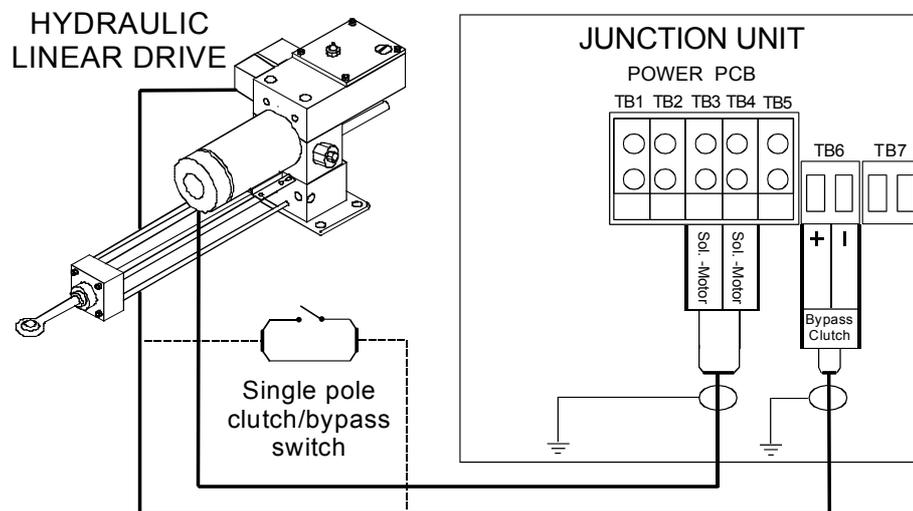
Figure 4-9 Connecting a hydraulic linear drive
