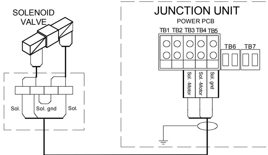
Figure 4-10 Connecting a solenoid valve
