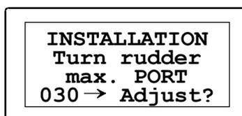
Manually turn the helm wheel to port until the rudder stops at maximum port rudder.
