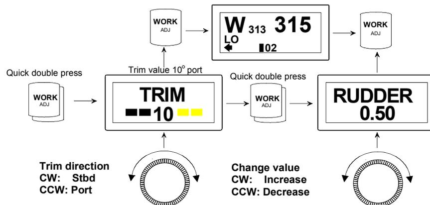
The LO (speed) parameters of Counter Rudder (C-RUDD) and Autotrim are automatically selected in WORK mode. The autotrim function and the Off-course alarm are controlled by speed input and are automatically turned off at speeds below 2 kts. If no speed input is provided the autotrim is permanently on and the Off-course alarm operates as in AUTO mode.
