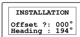
Dial in the correction by turning the course dial to offset the RFC35 heading to agree with the known, accurate heading. The offset value can be either positive or negative.
