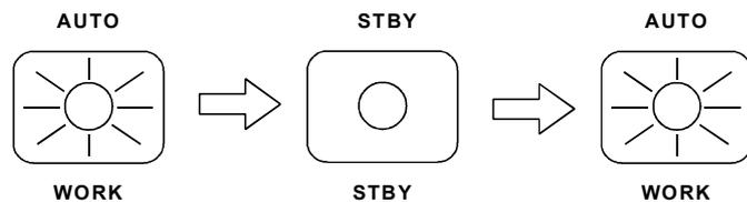
Operation of mode button returns the autopilot to initial mode.
