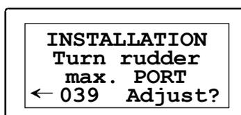
Adjust the displayed angle the same way as for starboard adjustment. (This time you need not correct for wrong side if the Rudder Feedback is upside down).
