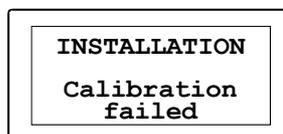
In that case move the compass to a better location and re-calibrate.
