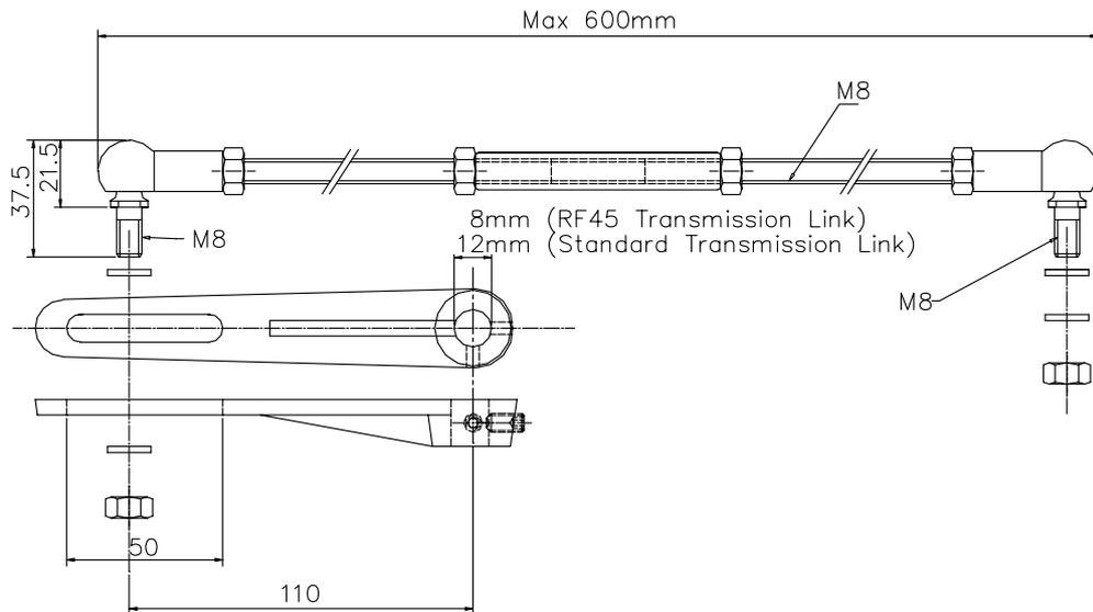
Figure 3-9 RF45 Transmission Link
