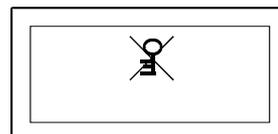
After having "unlocked" the other control stations, the "active" control unit will show the above symbol before the display returns to normal. All other control units will return to the "inactive" state.
