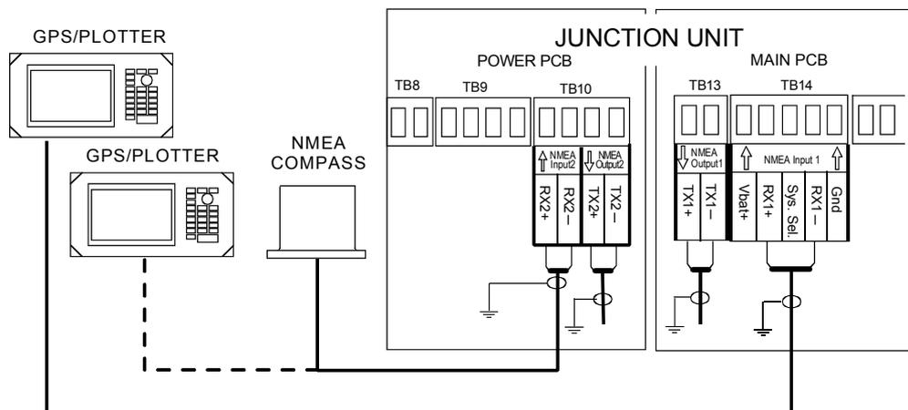
Figure 4-22 Double NMEA connection
