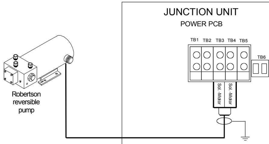
Figure 4-8 Connecting a reversible pump
