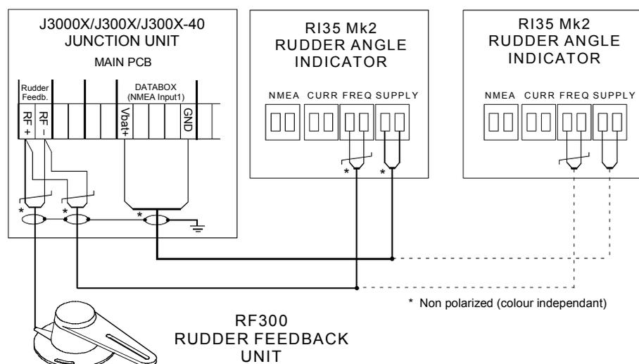
Figure 4-20 RI35 Mk2-J3000X/J300X Wiring diagram
