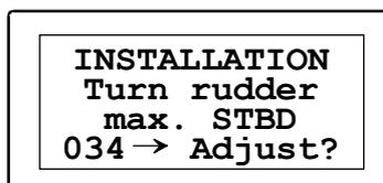
The value shown on the display is the value read by the feedback unit before any adjustment is made. The arrow indicates to which side the rudder is positioned. If the displayed angle is different from the actual angle, set correct rudder angle on the display by turning course selector clockwise to increase the value or counter clockwise to decrease the value.
