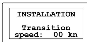
The transition speed is the speed where the AP35 will automatically change the steering parameter set from the HI speed to LO speed parameters, or vice versa.
