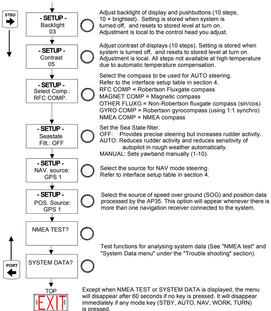
**Note !** *It is necessary to select the correct compass and Nav. source to make the autopilot operate.*
