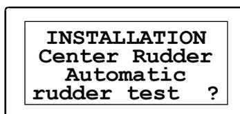
The display will alternate between Center Rudder and current rudder angle as long as the rudder is more than 10° out of midship.
