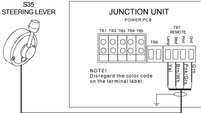
Figure 4-18 S35 connection to Junction unit
