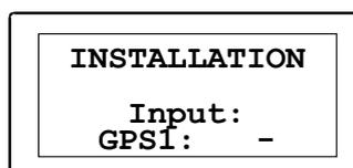
The display is now showing the first name on the list. Assign a hardware port to the name by turning the course selector until the hardware port is displayed.
