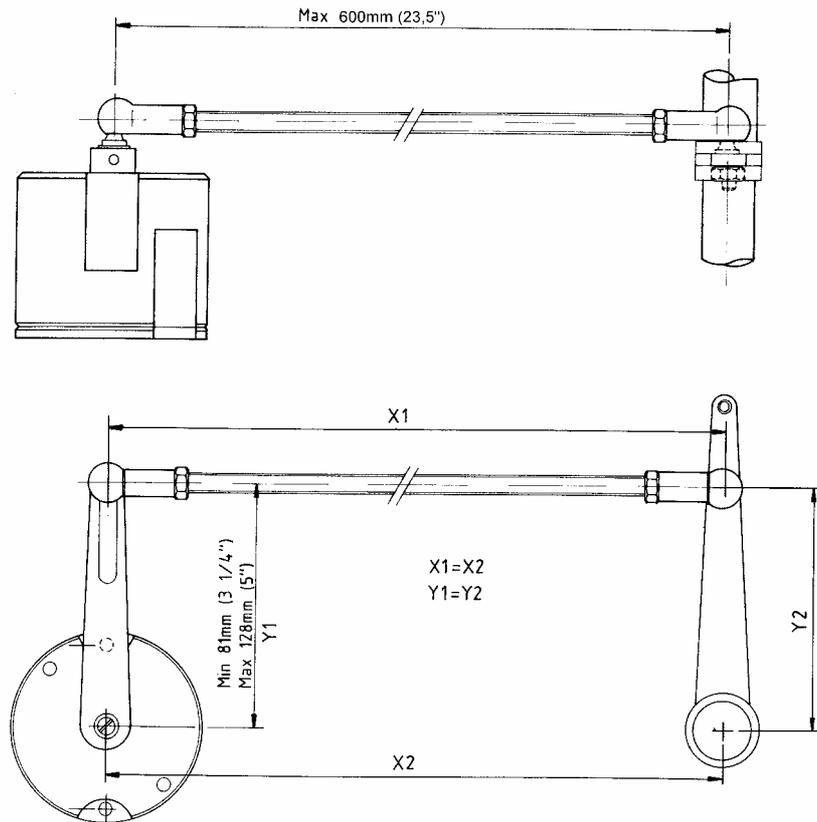
**Figure 4-4 RF45X Rudder Feedback Unit - Mounting**
