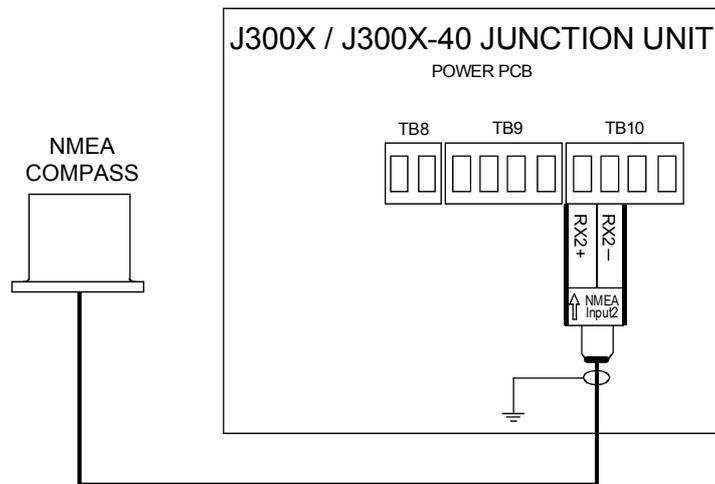
Figure 4-23 NMEA compass connection
