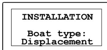
Actual boat type is selected by turning the rotary course selector. The options are: Displacement or Planing.
