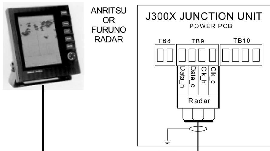
Figure 4-24 Radar Clock/Data connection
