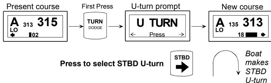
C-Turn changes the current set course continuously. The user may decide if the C-Turn should be made to Port or Starboard. C-Turn is activated by a second push on the TURN button, and can only be activated when the AP35 is in AUTO or WORK modes. The AP35 will continue on the set course until you press either the PORT or STBD button to select the direction to make the C-Turn. If you do not press PORT or STBD within 1 minute, the AP35 will return to the AUTO mode and stay on course.
